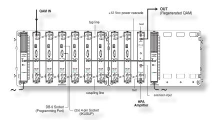
Example of CGT headend for eight QAM modulated channels.
